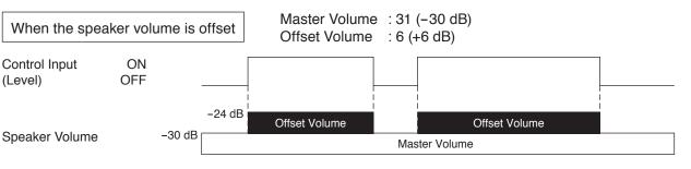
Offset Volume is applied while the Level signal is being received. Offset Volume is also applied to the audio of the ongoing broadcast in real time. This enables the audio volume control to be linked to the control input.
